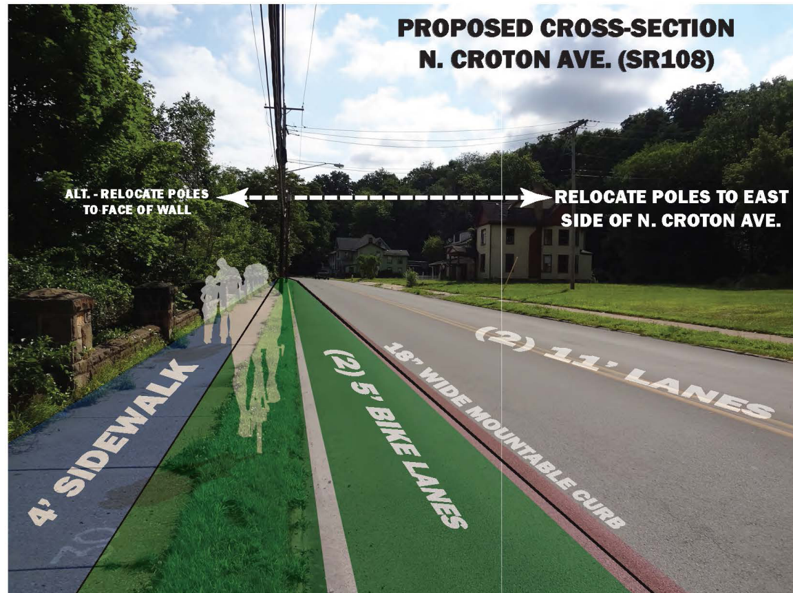
N. CROTON AVE. (SR108); ADT - 8,100; POSTED SPEED - 30MPH ROADWAY WIDTH, CURB TO CURB - 30'; 6' WIDE CONCRETE SIDEWALKS (BOTH SIDES OF ROAD) 8' DISTANCE FROM STONE WALL TO FACE OF CURB, SOUTHBOUND
